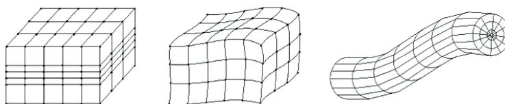
FIG. 5.2 – Examples of structured meshes.
